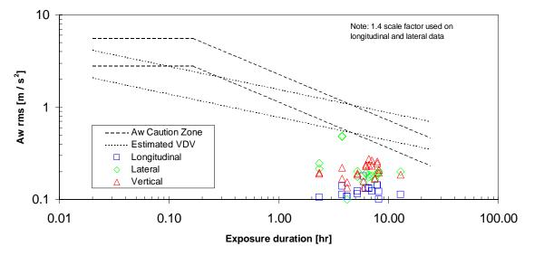
To put the locomotive vibration exposure level in perspective, the results were compared to the levels measured on heavy trucks, light and medium duty trucks, a van and a motorcycle. The locomotive vibration levels were also compared to levels reported for various vehicles found in the literature. The vibration environment on locomotives was found to be comparable to commercial on-road vehicles and below many commercial off-road vehicles and recreational vehicles.
