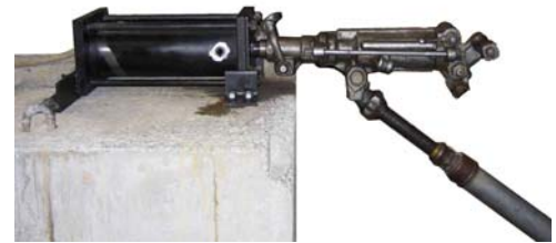
Figure 5. Jackleg drill (right) with the energy absorber (left)
