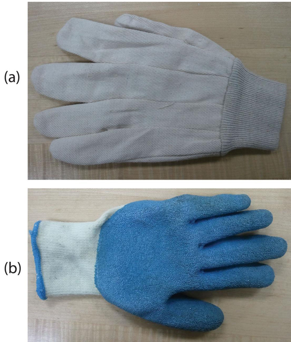
Figure 2. The polyester glove (a) and latex glove (b) are commonly used at workplaces to protect workers' hand. These gloves can change the coefficient of friction at the hand-handle interface.
