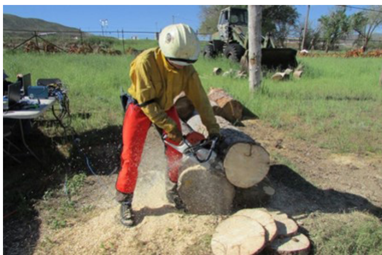
Figure 1. Sawyer cuts slices from logs while the vibration is measured at the hand-handle interface. Photo by NIOSH.
