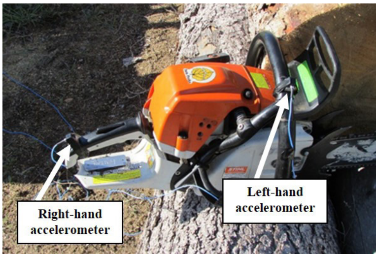
Figure 2. White arrows point to the two tri-axial accelerometers used to measure the acceleration at the hand-handle interface for right hand (rear handle) and the left hand (front handle). Photo by NIOSH.
