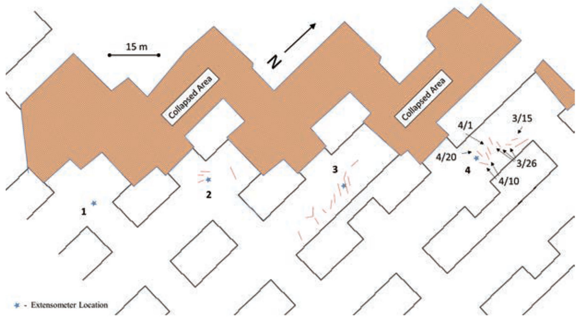
Figure 1 - Extensometer locations, shown as blue stars, along with crack locations and orientations, shown as red lines, and the dates they were first observed.
