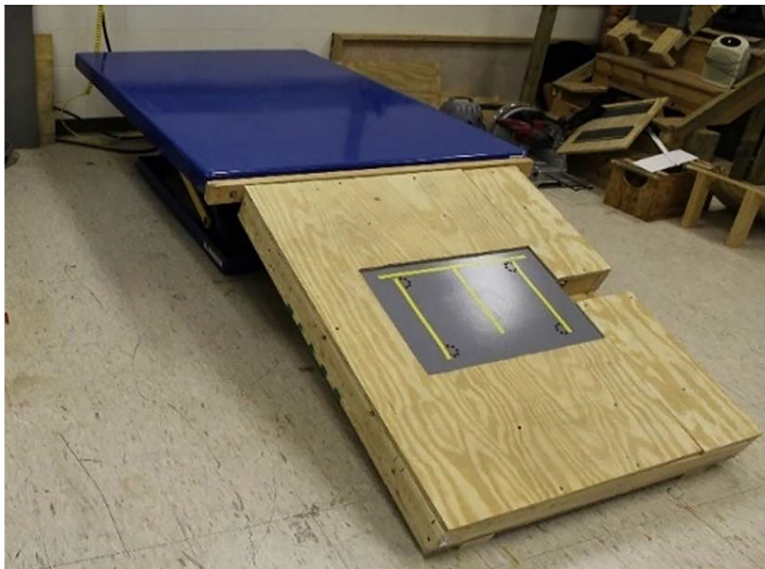
Fig. 3. Wooden roof platform elevated by hydraulic lift
