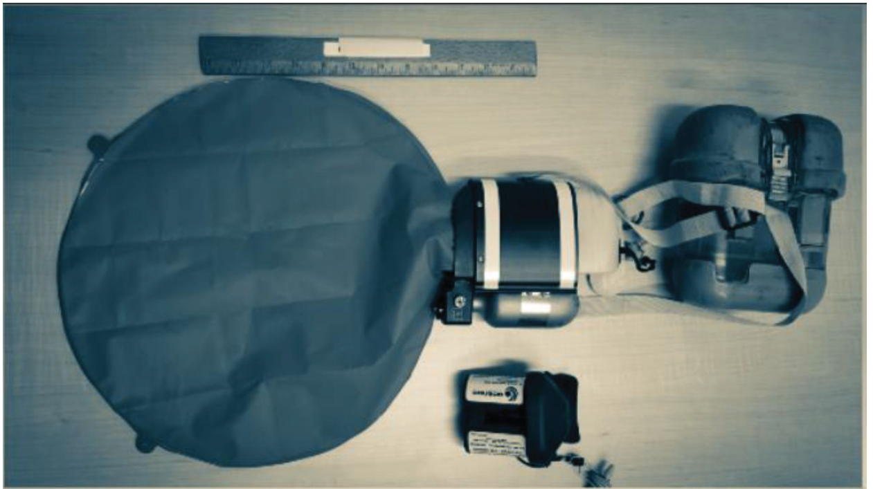
FIGURE 1. (TOP) A 10-MINUTE DURATION SCSR UNIT (LEFT) AND CARRYING CASE (RIGHT); (BOTTOM) SCSR SIMULATOR EXPECTANCY TRAINING DEVICE. A 12- INCH RULER IS PROVIDED FOR SCALE
