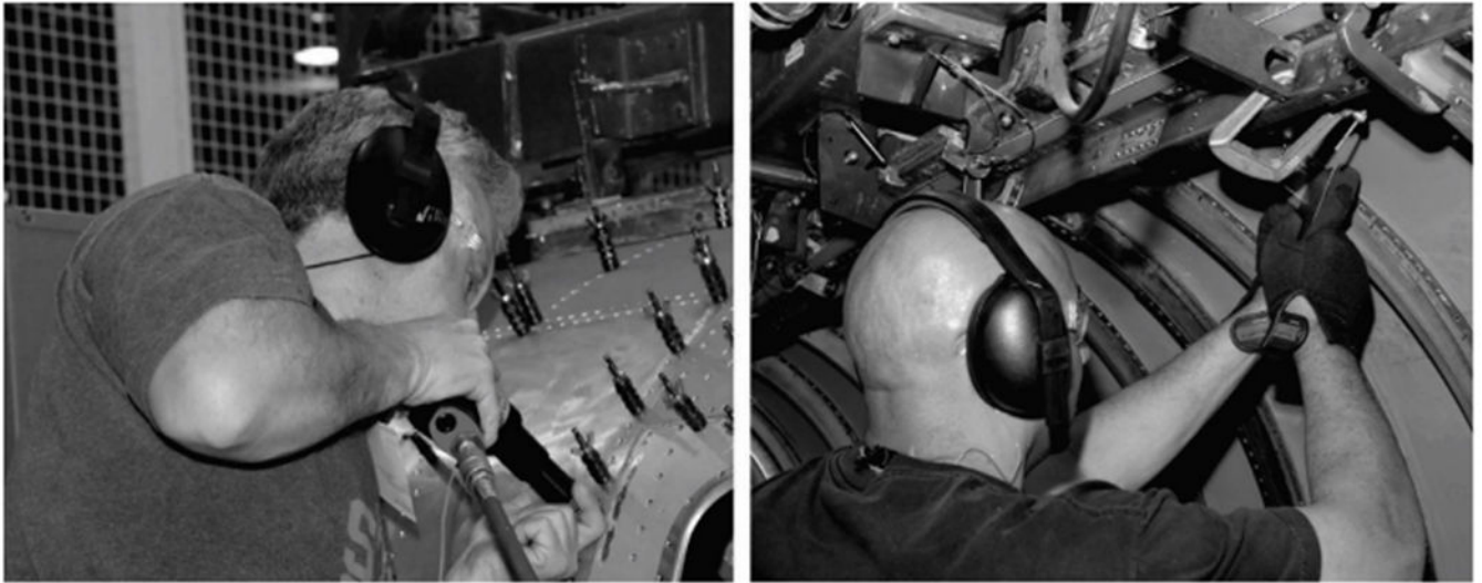
Fig. 1. Manual percussive riveting of aircraft sheet metal skins requires two riveting tool operators; one worker operates the riveting hammer (left) on the exterior surface of the assembly, while a second worker operates the bucking bar (right) on the interior of the airframe. The riveting hammer delivers a rapid series of impacts while the bucking bar supplies the opposing force. The metal rivet is mechanically deformed and work-hardened between the two riveting tools to securely fasten the sheet metal to the airframe.
