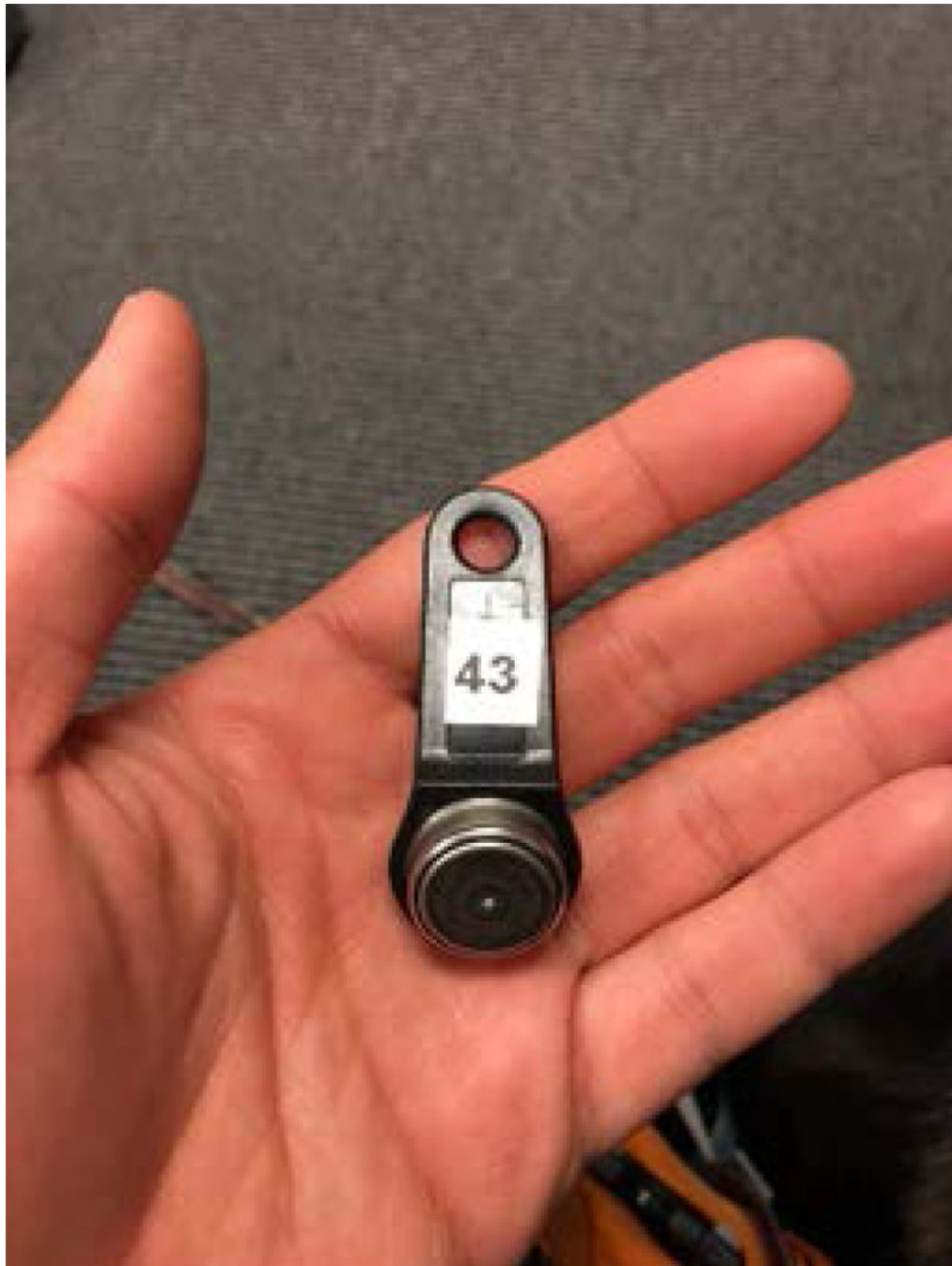
Figure 1. Photo of an iButton. Pictured here is a Maxim iButton in the palm of a hand for scale.
