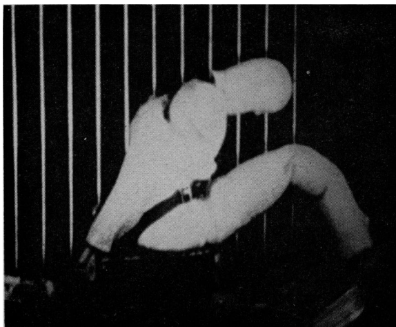
Figure 6. Limit of forward motion in 21 mph impact, using a combination lap and chest strap, floor-anchored
