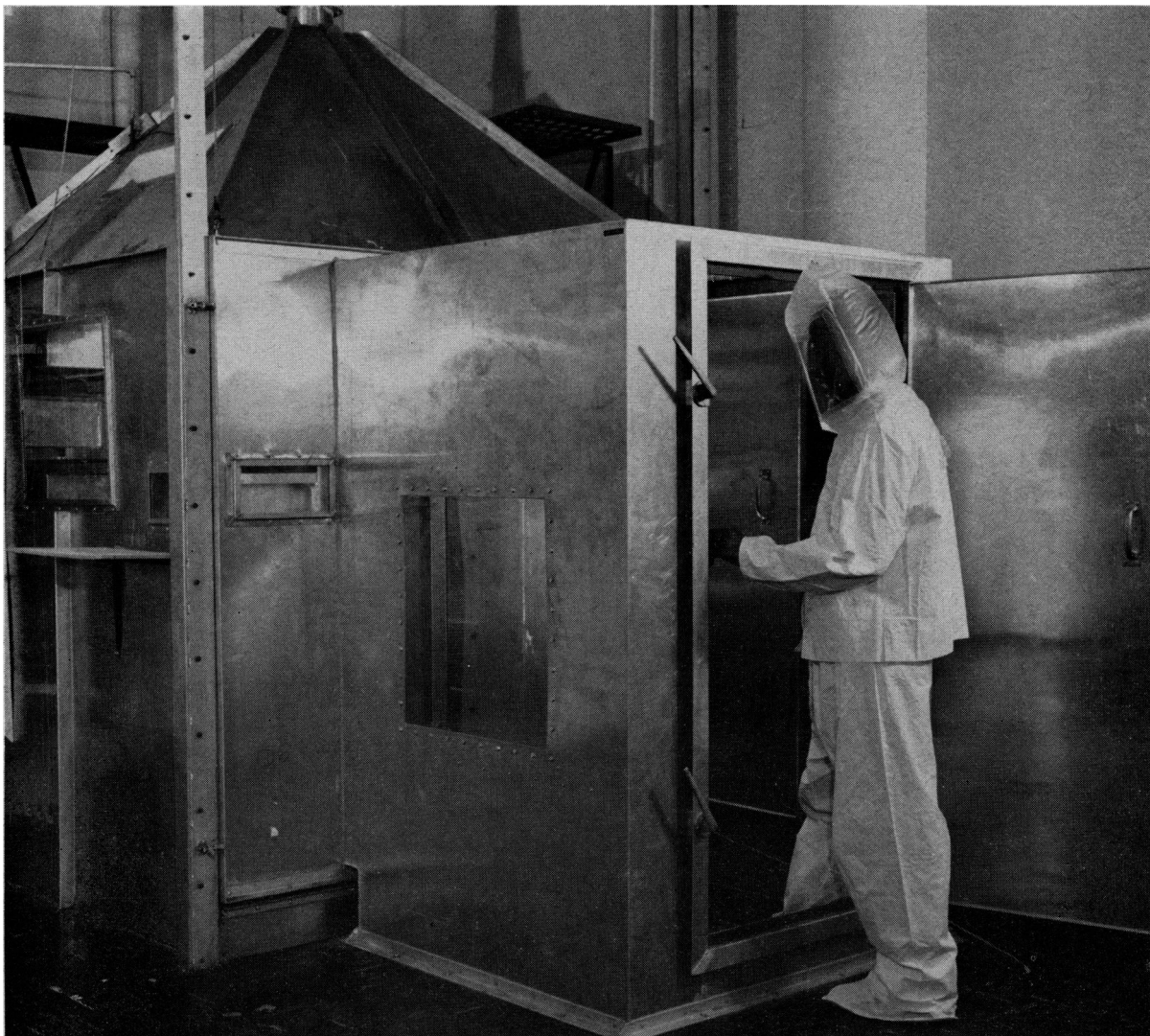
Animal inhalation exposure chamber used for the study of highly toxic airborne industrial chemicals
