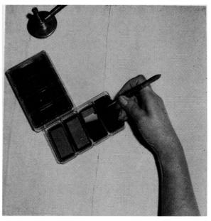
Figure 2. Plating a filter paper strip
