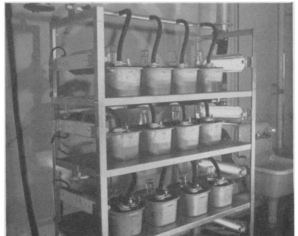
Figure 6. Filtered air is supplied to individual cages connected to negative pressure manifold.
