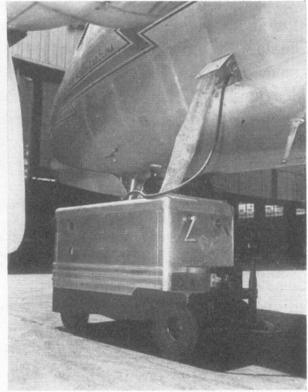
Left: Compact toilet room. Above: External servicing panels with waste water valve and drain (left) and sewage outlet, flushing water inlet, and valve. Right: Large hose drains sewage into cart beneath plane. Small hose pumps flushing water and deodorant into toilet.
