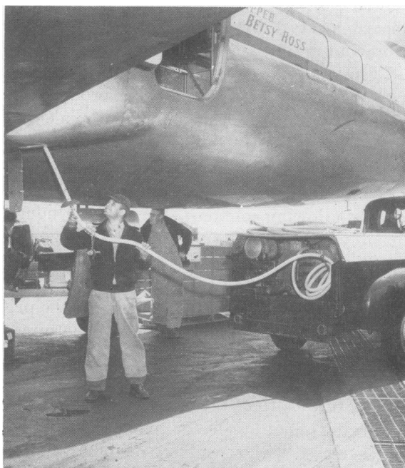
Filling an aircraft water system at stopover point.
