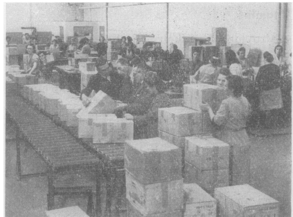
The depot was capable of sorting, reconditioning, and repacking 600,000 cans per 48-hour working week with a staff of 150, mainly women. The average output was 4,000 cans per man-week.
