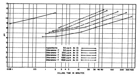
Figure 1. Effect of pH and concentration of chloramine-T on killing time (99.9999 percent) of *Micrococcus pyogenes* var. aureus:25° C.
