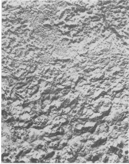
FIGURE 9.—Heavily discolored opaque area, 130 X.
