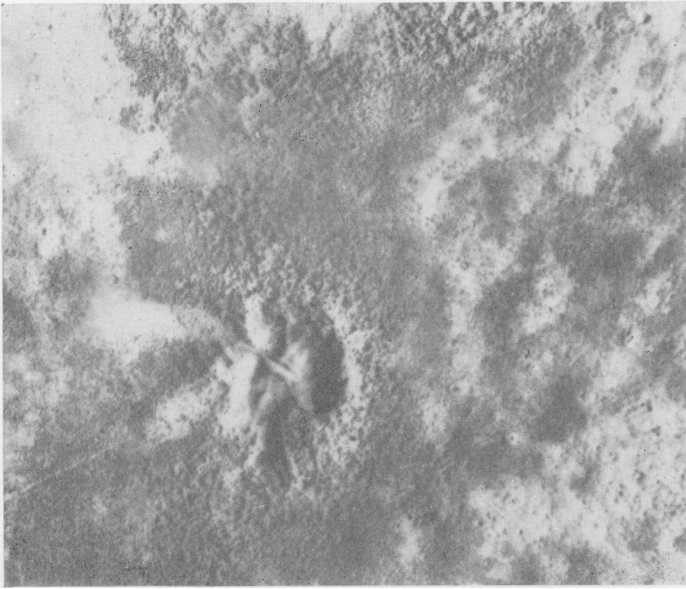
FIGURE 11.—Small pit in opaque-white surface, 150 X.
