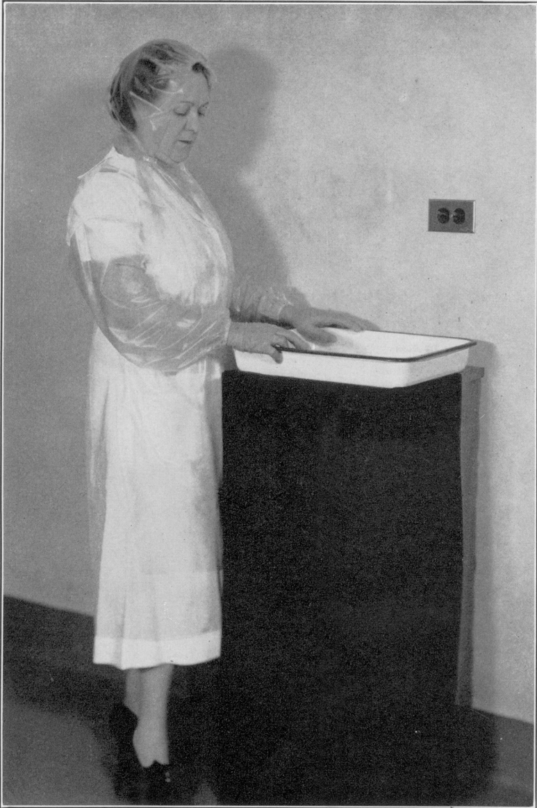
FIGURE 2. —Protective hood, sleeves, gloves, and apron. Note sleeves secured over gloves, neck protected by hood, and apron extending to neck.
