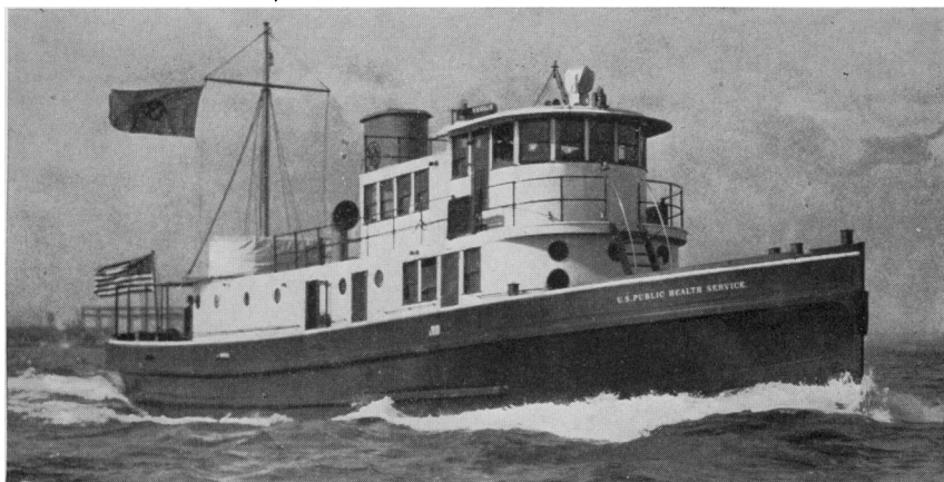
New Diesel-electric powered boarding vessel for quarantine stations in northern waters.
