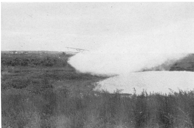
FIGURE 6.—Huff-Daland dusting plane, treating Harris Station experimental pool, Wheeler Reservoir. Altitude 10 feet.
