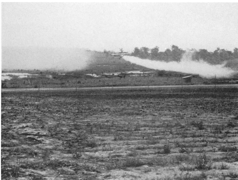
FIGURE 8.—Stearman dusting plane, treating a swamp near Muscle Shoals airport. Note dust cloud in left background which was laid down just previous to cloud in process of liberation.
