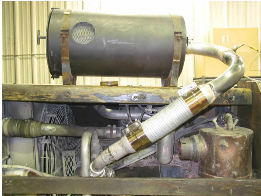
Figure 3.—Filtration system used in testing high-temperature disposable elements from Donaldson and Filter Service.
