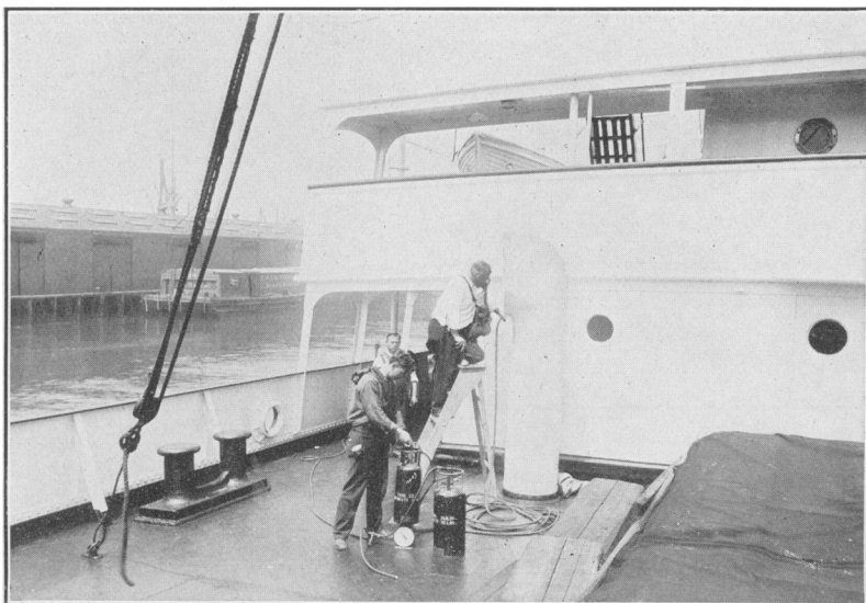
FIGURE 5.—Air jet sprayer in use on a loaded ship. The air line from the fumigating boat is connected with the air tank
