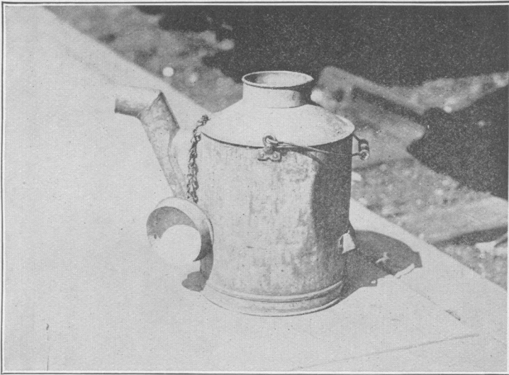
B. Water pail with protected nozzle and cover used for filling water coolers. A pail of excellent design.
