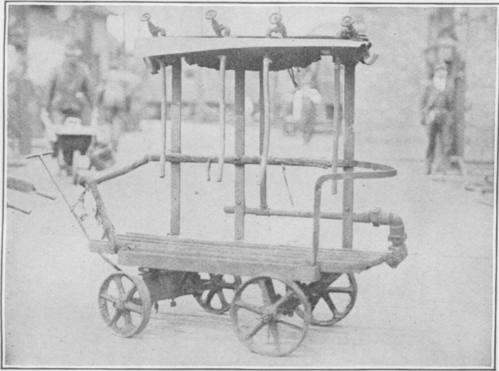
A. A portable steam sterilizing truck used in the C., M. & St. P. coach yard in Chicago.
