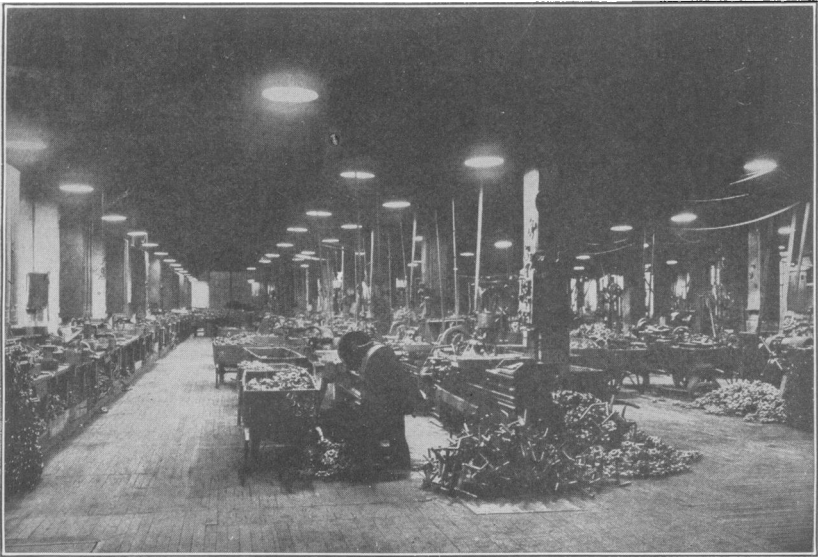
Fig. 11.—In this well-lighted machine shop note the even distribution of light and freedom from glare. The illumination is economically concentrated on the work. As it appears in the illustration, additional light on the ceiling would render the room more cheerful.
