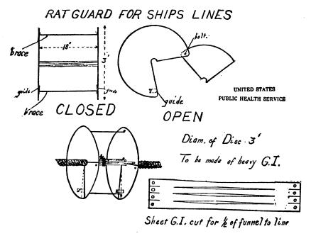
After closing the guard over a ship's line, the central part of the funnel is tied to the line by a small piece of rope. This fastens the rat guard to the ship's line so that it can not slip and completely closes the funnel and locks the two halves of the rat guard.
