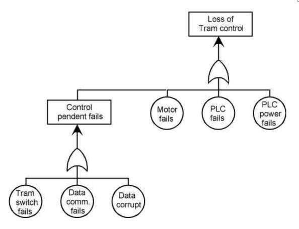
Figure 20.—Fault tree for the loss of tram control hazardous event.
