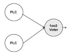
Figure 9.—A redundant PLC architecture.
