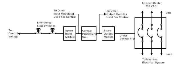
Figure 24.—Conceptual diagram of a PLC-based safety system that shares a 1001 industrial PLC used for machine control.
