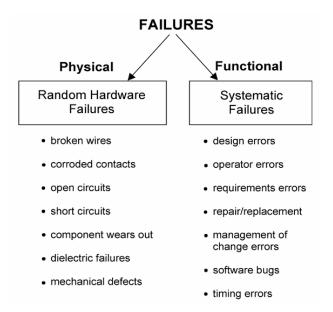
Figure 12.—Failure classifications.
