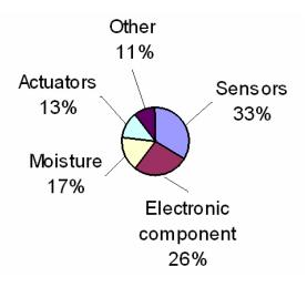
Figure 15.—Random failures for 100 PE-based mining system mishaps during 1995–2001.
