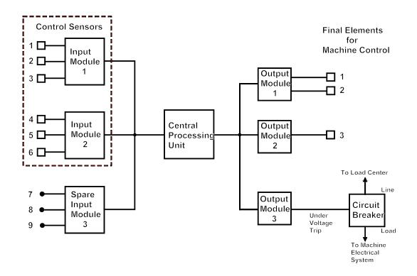
Figure 23.—A 1001 industrial PLC used for machine control.
