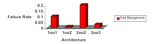
Figure 10.—Dangerous failure rates for various switch architectures.
