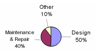
Figure 14.—Systematic failures for 100 PE-based system mishaps during 1995–2001.
