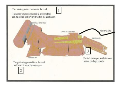
Figure 18.—A continuous mining machine.
