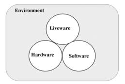
Figure B–1.—The SHEL model of a system.
