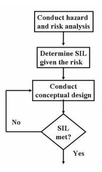
Figure 7.—The general design process to attain the required SIL.
