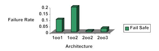
Figure 11.—Safe failure rates for various switch architectures.
