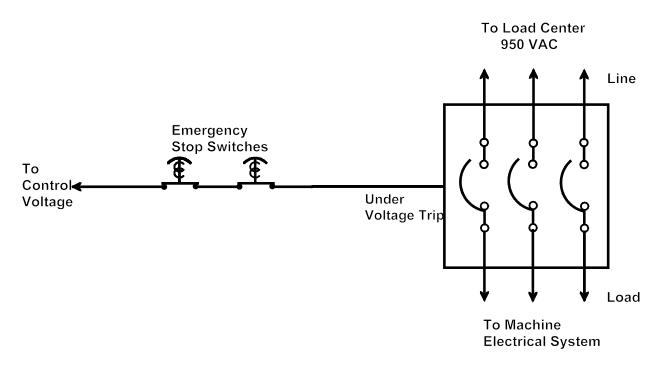
Figure 22.—Emergency stop system using lower failure rate switches.
