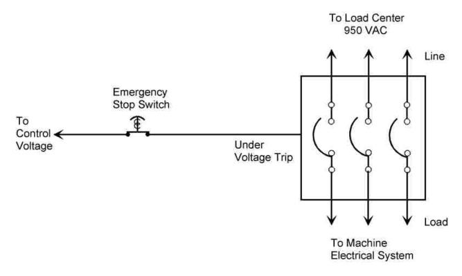
Figure 21.—Emergency stop system using a single, generic switch.
