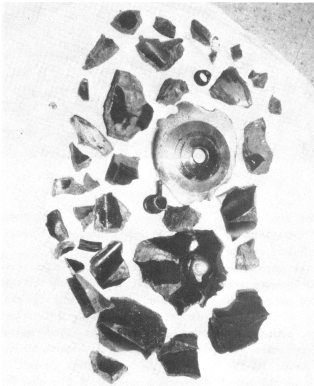
Figure 6. Pieces of exploded rotor removed after decontamination
