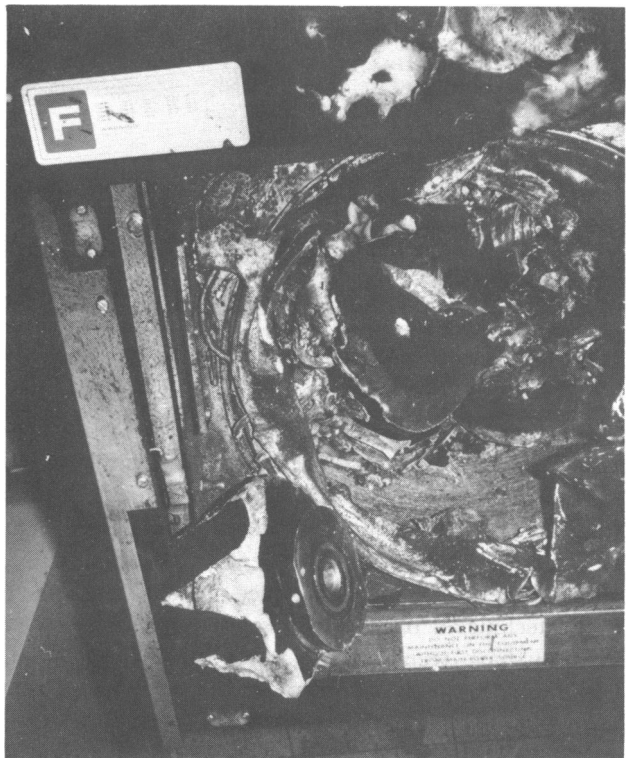
Figure 7. Base of rotor, with overspeed safety pin removed, and centrifuge chamber
