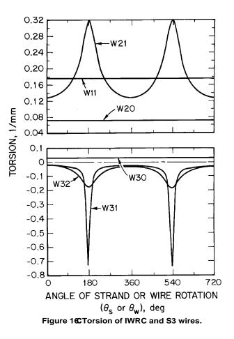
deformations in the geometry of the rope structure needs to be determined. The major change is axial elongation along the centroidalaxis of a wire. Accompanying the axial elongation is a lateral contraction of the cross section. In addition, bendingand twisting moments are generated in the wire that cause changes in the curvature and torsion of the wire. The combination of all of these individual wire deformations results in the deformation of the rope structure.
