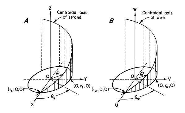
Figure 4C Coordinate systems for single helix.A, rope coordinate systemB, strand coordinate system.
