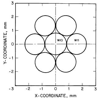
Figure 6.CStrandarrangement of 33-mm 6×19 Seale, IWRC, right regular lay wire rope.
