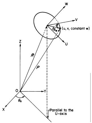
Figure 5 Coordinate system for double helix.
