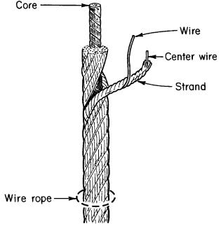
Figure 1 CStructural elements in a typical wire rope.
