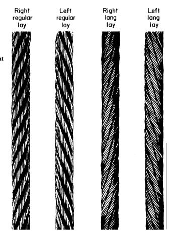
Figure 2.C Comparison of typical wire rope lays.
