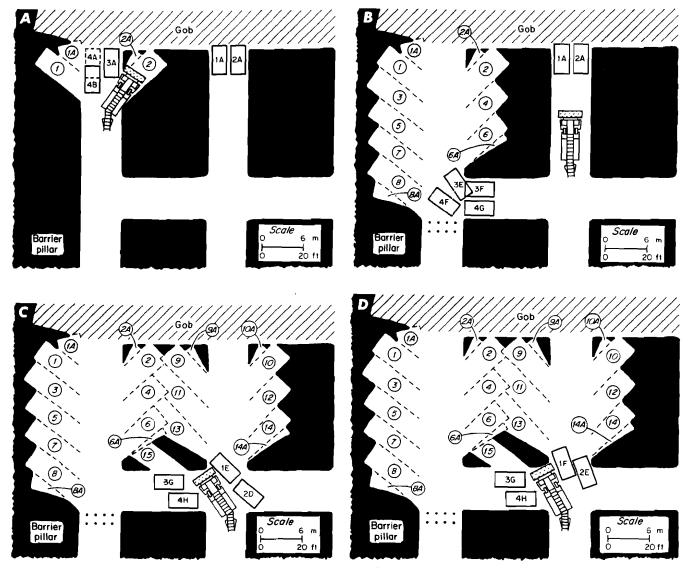
Figure 2.—Christmas tree extraction method. *A*, lifts 1-2A. *B*, lifts 1-8A. *C*, lifts 1-push; pushout removal with units 1 and 2 in tandem. *D*, lifts 1-push; pushout removal with units 1 and 2 staggered.
