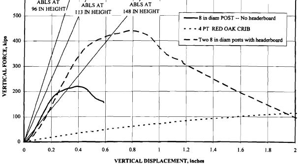
Figure 31.—Comparison of support stiffness with that of conventional timber posts. *A*, Fletcher support; *B*, VAMT support.
