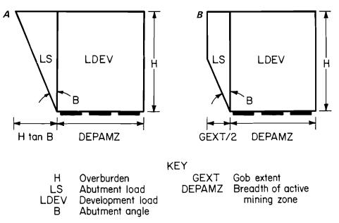
Figure 5.—Schematic showing the abutment load in two dimensions. *A*, supercritical gob; *B*, subcritical gob.
