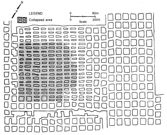
Figure 1.--Failed split-pillar workings in Mine A.
