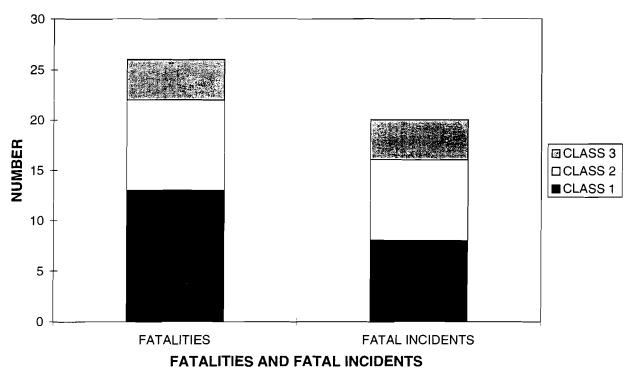
Figure 10.—Fatal roof/rib incidents and fatalities associated with retreat mining, 1989-96.
