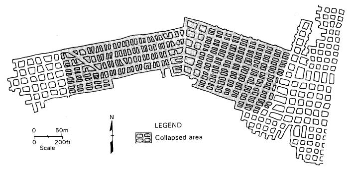
Figure 2.—Location of split-pillar collapse at Mine C.
