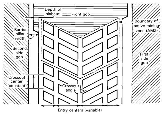
Figure 1.—Section layout parameters used in ARMPS.
