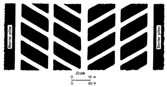
Figure 8.—Three-way intersection belt entry design.
