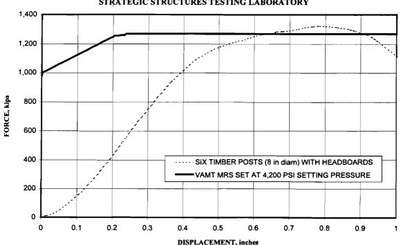
MOBILE ROOF SUPPORT TESTS STRATEGIC STRUCTURES TESTING LABORATORY
