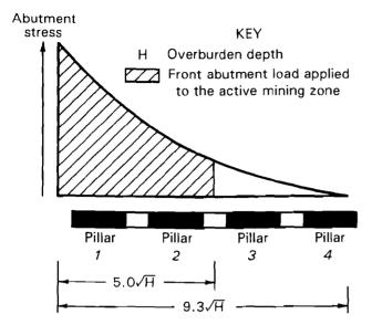
Figure 4.—Distribution of abutment stress, showing that 90% of the abutment falls within the distance of  $(5\sqrt{R})$  from the gob edge.
