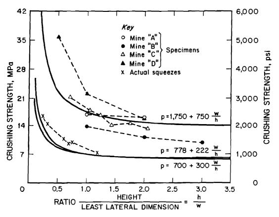
Figure 1.--Data used to develop the first U.S. pillar strength formula (after Bunting, [1911]).
