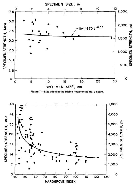
Figure 8.—Specimen strength and HGI of U.S. coalbeds.
