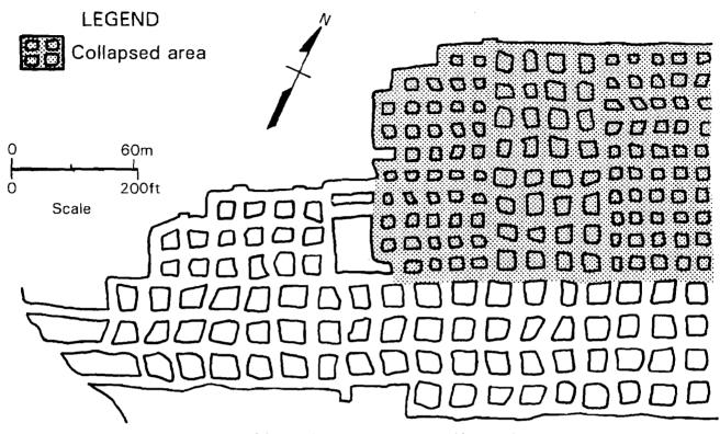
Figure 3.---Failed small-center development workings at Mine D.
