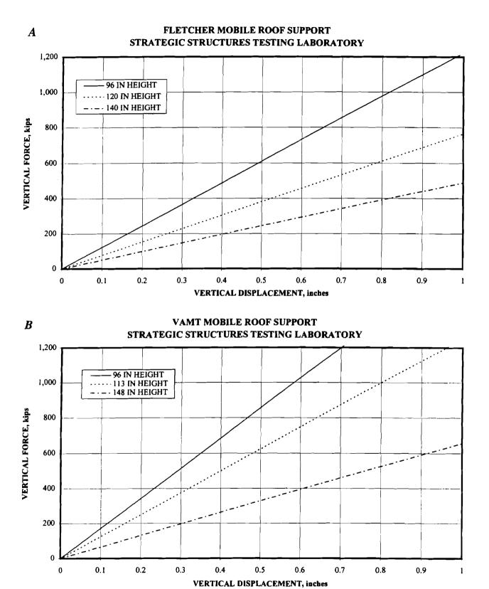
Figure 7.—Effect of support height on vertical stiffness. *A*, Fletcher support; *B*, VAMT support.
