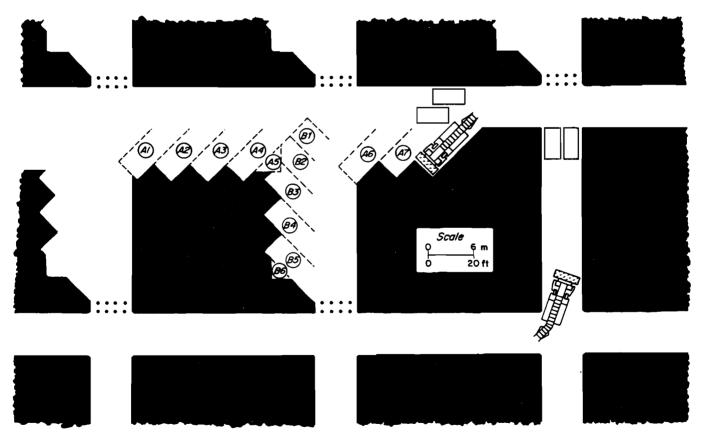
Figure 9.—Partial pillar extraction by slabbing.
