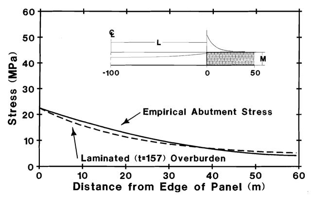
Figure 3.---Plot of the laminated abutment stress fitted to the empirical formula.
