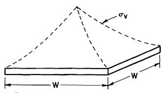
Figure A-2.—Determination of pillar load-bearing capacity as the integral of the pillar stress distribution.
