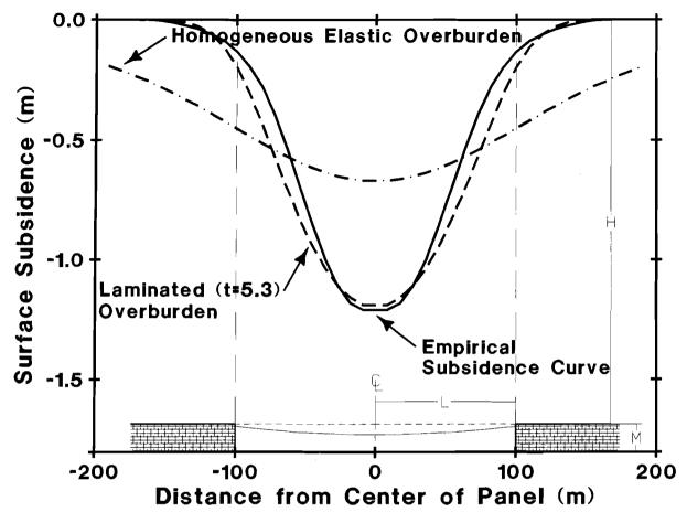
Figure 6.—Plot of the laminated and homogeneous isotropic subsidence fitted to the empirical curve.
