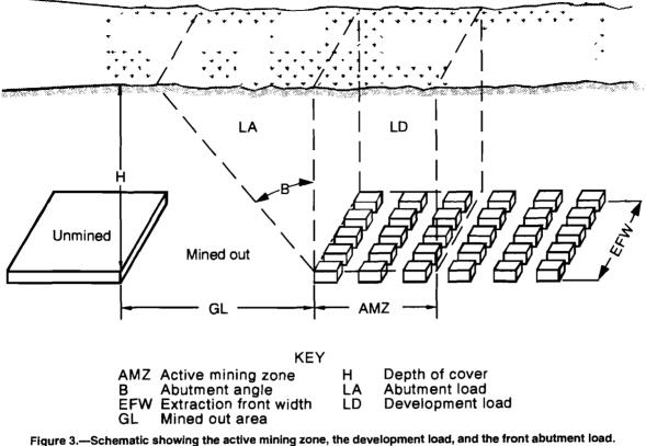
The AMZ includes all of the pillars on the extraction front (or "pillar line") and extends outby the pillar line a distance of five times the square root of the depth of cover  $(5\sqrt{H})$ . This distance was selected because measurements of abutment stress distributions [Mark 1990] show that 90% of the front abutment load falls within its boundaries (figure 4).
