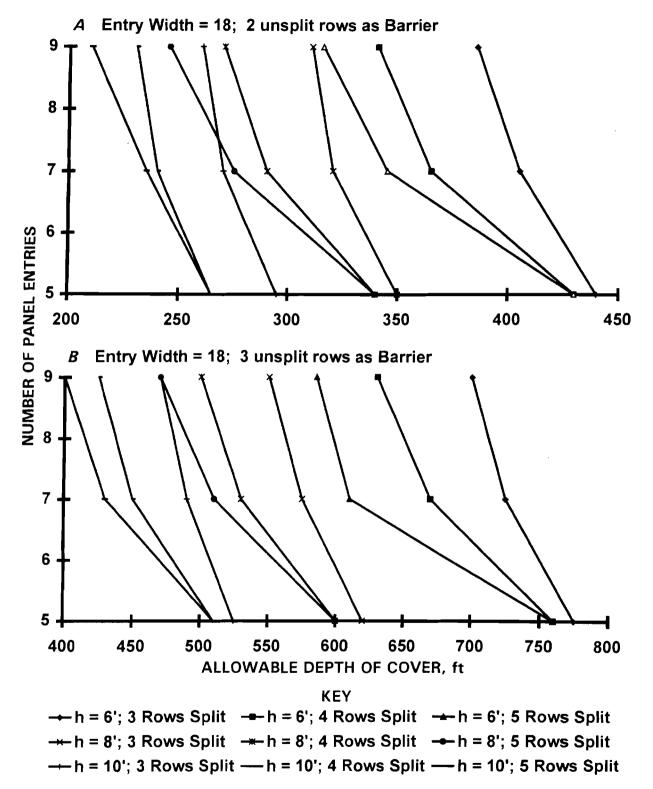
Figure 9.—*A*, suggested maximum depth for two rows of unsplit pillars as barrier between gob areas, 5.5-m (18-ft) entry, 18by 18-m (60- by 60-ft) pillars. *B*, suggested maximum depth for three rows of unsplit pillars as barrier between gob areas, same entry and pillar sizes.
