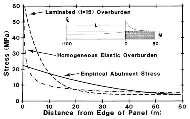
Figure 2.—Comparison of longwall abutment stress computed from the laminated and homogeneous isotropic models and from the empirical formula.
