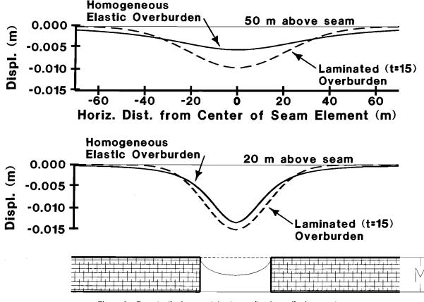
Figure 4.—Remote displacement due to a unit volume displacement.
