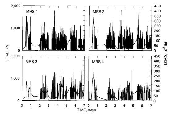
Figure 6.—Total loads on mobile roof supports.
