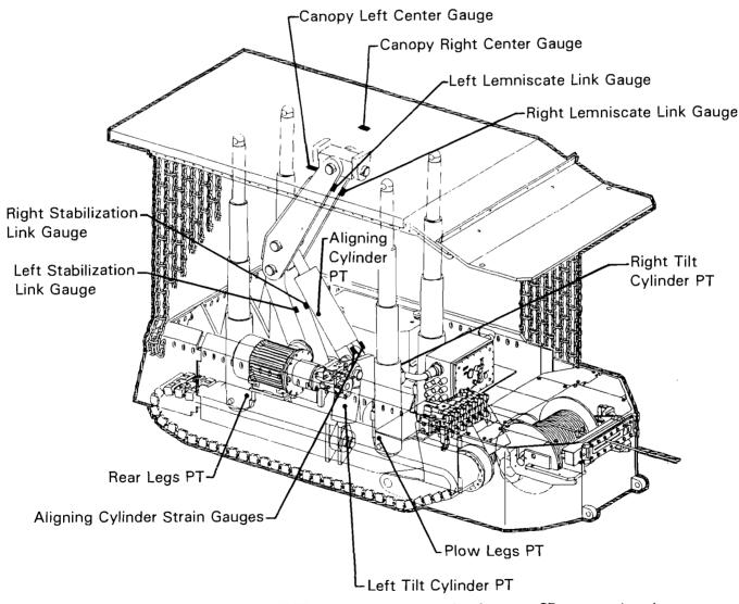
Figure 3.—Instrumentation installed on the VAMT support to assess support performance. PT = pressure transducer.
