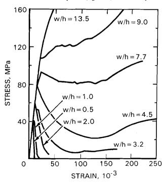
Figure 4.—Complete stress-strain curves for Indian coal specimens, showing increasing residual strength with increasing w/h ratio (after Das [1986]).
