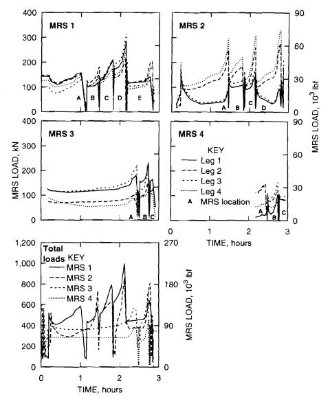
Figure 4.—Loading patterns on mobile roof supports.
