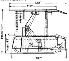
Figure 5.—Tilt-frame lemniscate assembly utilized on the VAMT support.
