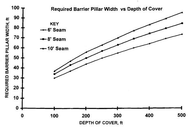
Figure 10.—Suggested solid coal barrier width between two areas where pillars have been split.
