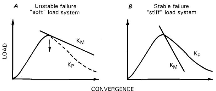
Figure 6.—Illustration of the local mine stiffness concept. *A*, local mine stiffness ( $K_m$ ) is less than postfailure stiffness of the pillar ( $K_p$ ), resulting in unstable failure. *B*, local mine stiffness ( $K_m$ ) exceeds the pillar's postfailure stiffness ( $K_p$ ), resulting in slow and stable failure.
