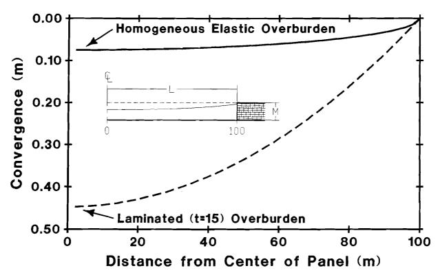
Figure 1.—Comparison of longwall convergence computed from the laminated and homogeneous isotropic models.
