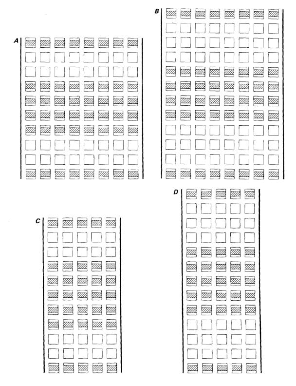
Figure 8.—Possible pillar-splitting plan for airblast control. *A*, nine-entry system, two rows of unsplit pillars for barrier. *B*, nine-entry system, three rows of unsplit pillars for barrier. *C*, six-entry system, two rows of unsplit pillars for barrier. *D*, six-entry system, three rows of unsplit pillars for barrier.
