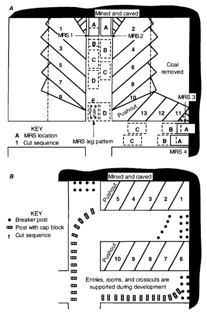
Figure 3.—Mining plan using (A) mobile roof supports and (B) posts.
