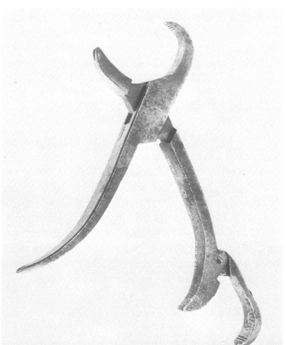
Figure 13. A double-ended dental pelican, made around 1800. This tool for extracting teeth has changed little over the years. Smithsonian collection
