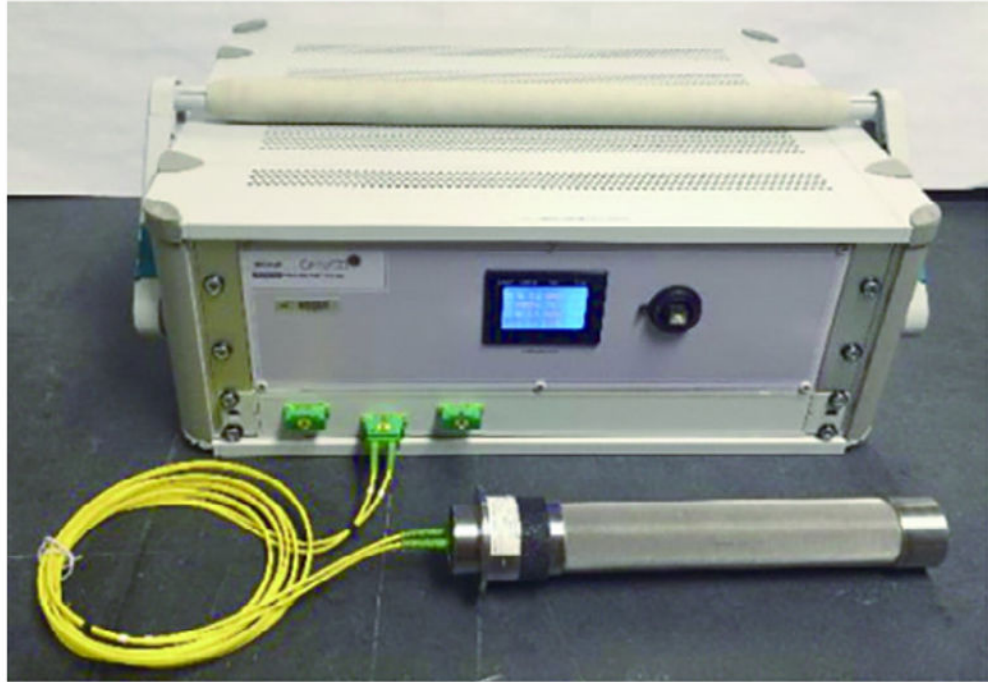
Fig. 1. RSL fiber optic methane detection system.
