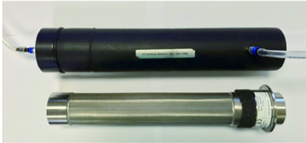
Fig. 6. Cylindrical tube and fiber optic sensor.
