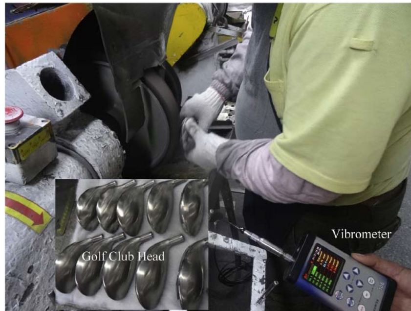
Fig. 1. A worker is grinding a golf club head at a typical workstation with a belt grinding machine (with a large drive wheel) in a sport equipment manufacturer.
