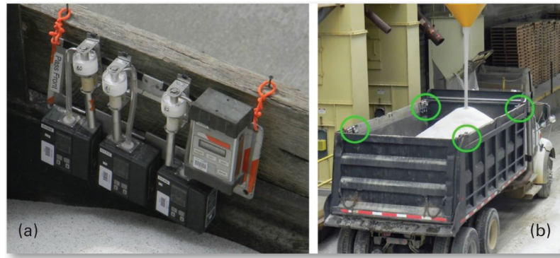
Figure 4. (a) Gravimetric and pDR sampling rack, and (b) sampling locations on truck at plant A.
