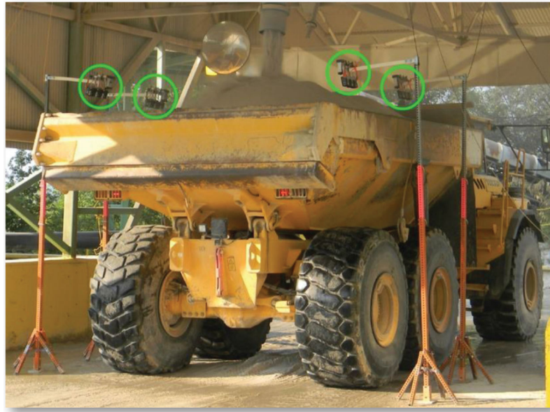
Figure 5. Adjustable sampling stands and sampling racks positioned around mine truck at plant B.
