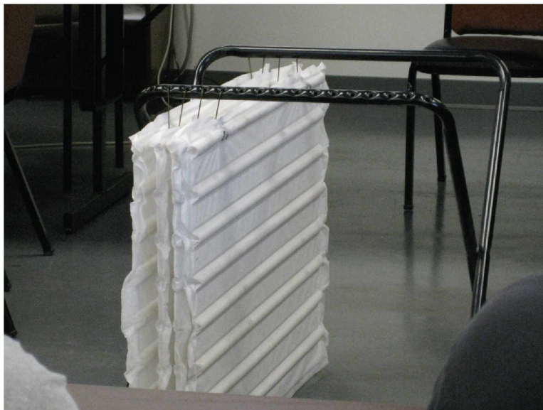
Figure 3. Mock-up of scrubber curtains and the stand used to hold them.
