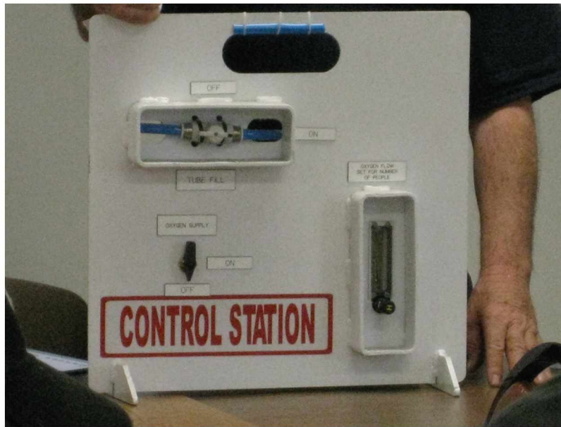
Figure 4. Mock-up of the internal oxygen controls and gauges on a refuge chamber.
