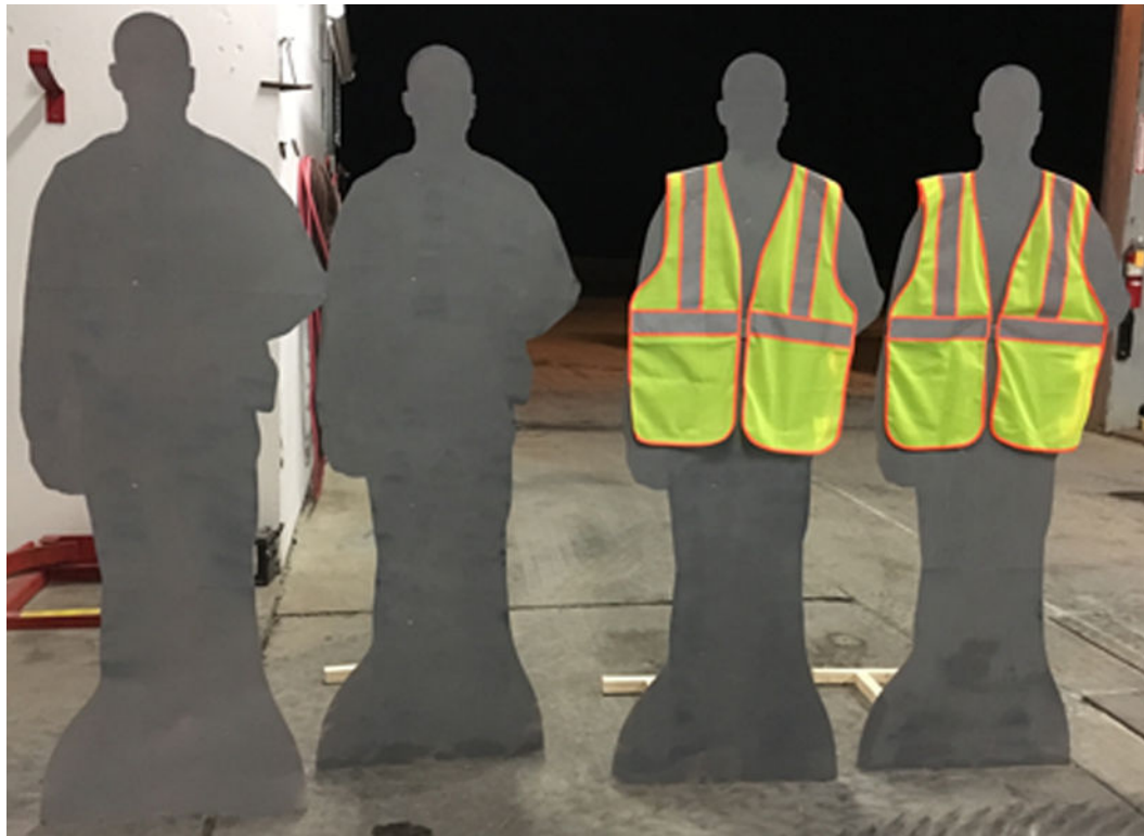
Figure 2. Cardboard Cut-outs Used to Simulate Workers.
