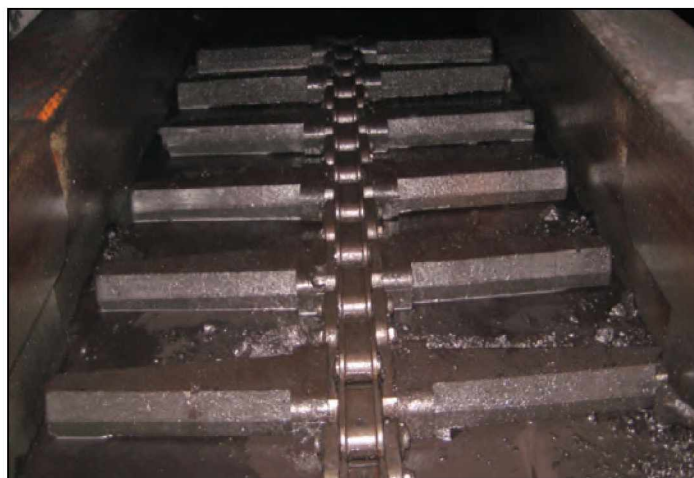
Figure 1.—Urethane-coated flight bar chain used in the conveyor system for a continuous mining machine.
