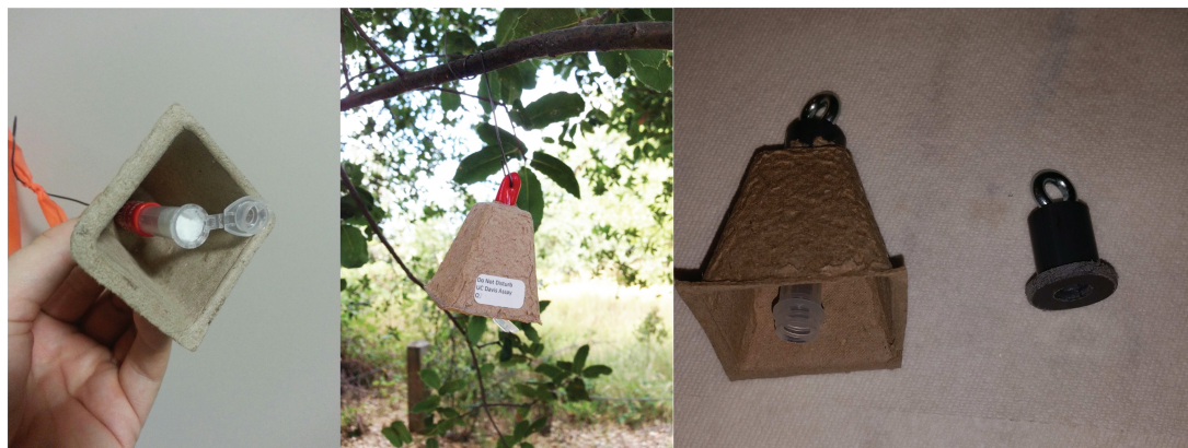
Fig. 1. Photographs of sugar baits. Sugar bait devices were constructed by threading baling wire through a caulking cap and feeding it through the hole of a seedling starter pot. A 2-ml plastic tube (Eppendorf) was filled with ~2 ml of a 40% sucrose and tap water solution and plugged with a cotton dental wick, and this bait tube was inserted into the open end of the caulking cap. Once deployed, the sugar soaked cotton wick was exposed for sugar seeking mosquitoes to access for 6 to 7 d. The image on the right compares the peat pot cover used in SAYO Counties to the small PVC cover used in the COAV.
