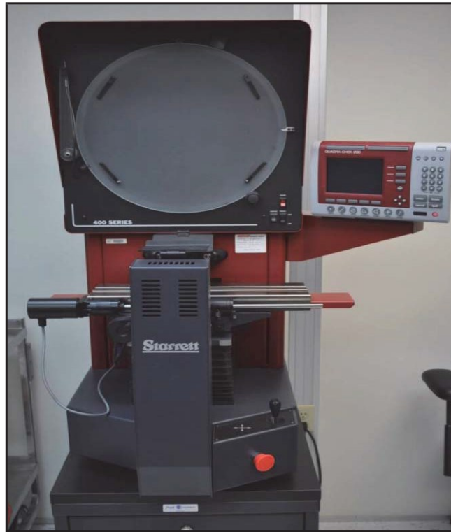
Figure 2-16. NIOSH Optical Thread Comparator
