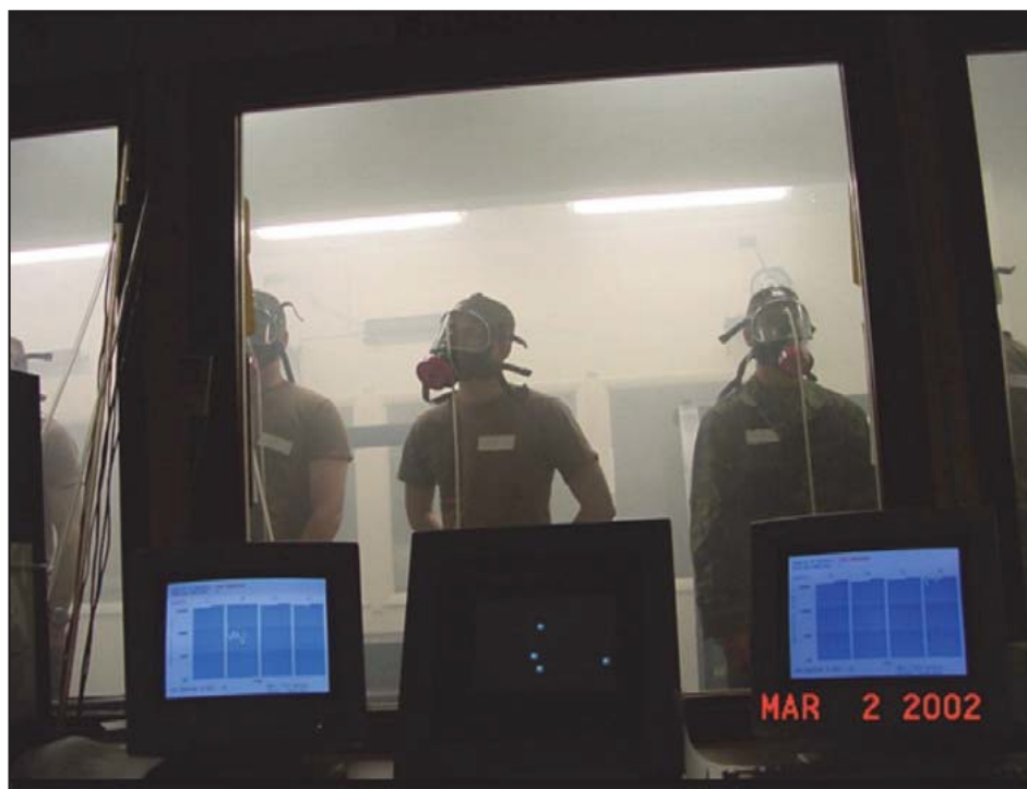
Figure 2-7. LRPL Test Chamber
