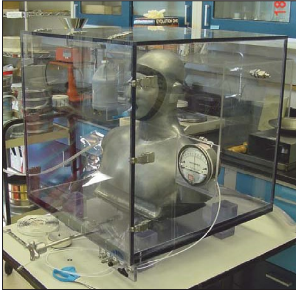
Figure 2-5. Live Agent Test Chamber
