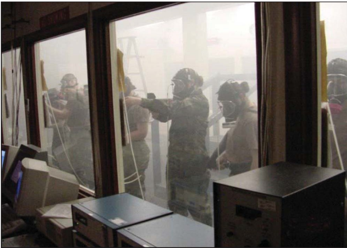
Figure 3-13. CBRN Respirator LRPL Testing
