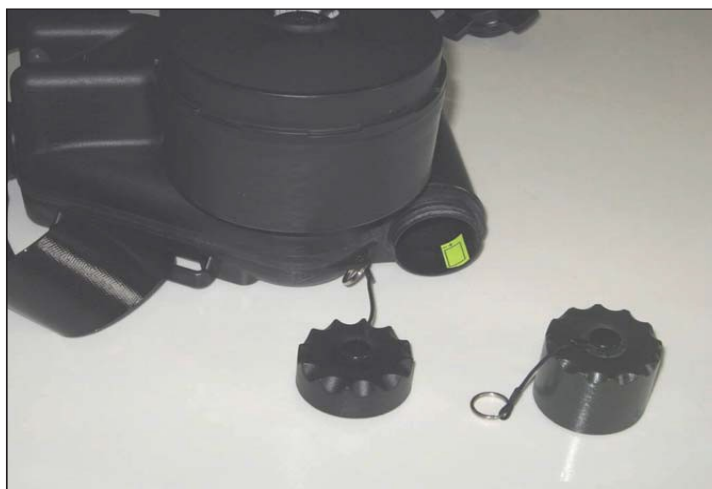
Figure 3-21. This NIOSH approved CBRN PAPR blower can be operated with different types of batteries. To identify the type of battery to be used, manufacturers supply battery covers of different colors or lengths. This picture shows the short cover for non-rechargeable batteries and the longer cover for rechargeable batteries.
