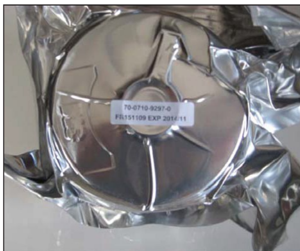
Figure 3-8. CBRN Canister Shelf Life Label
