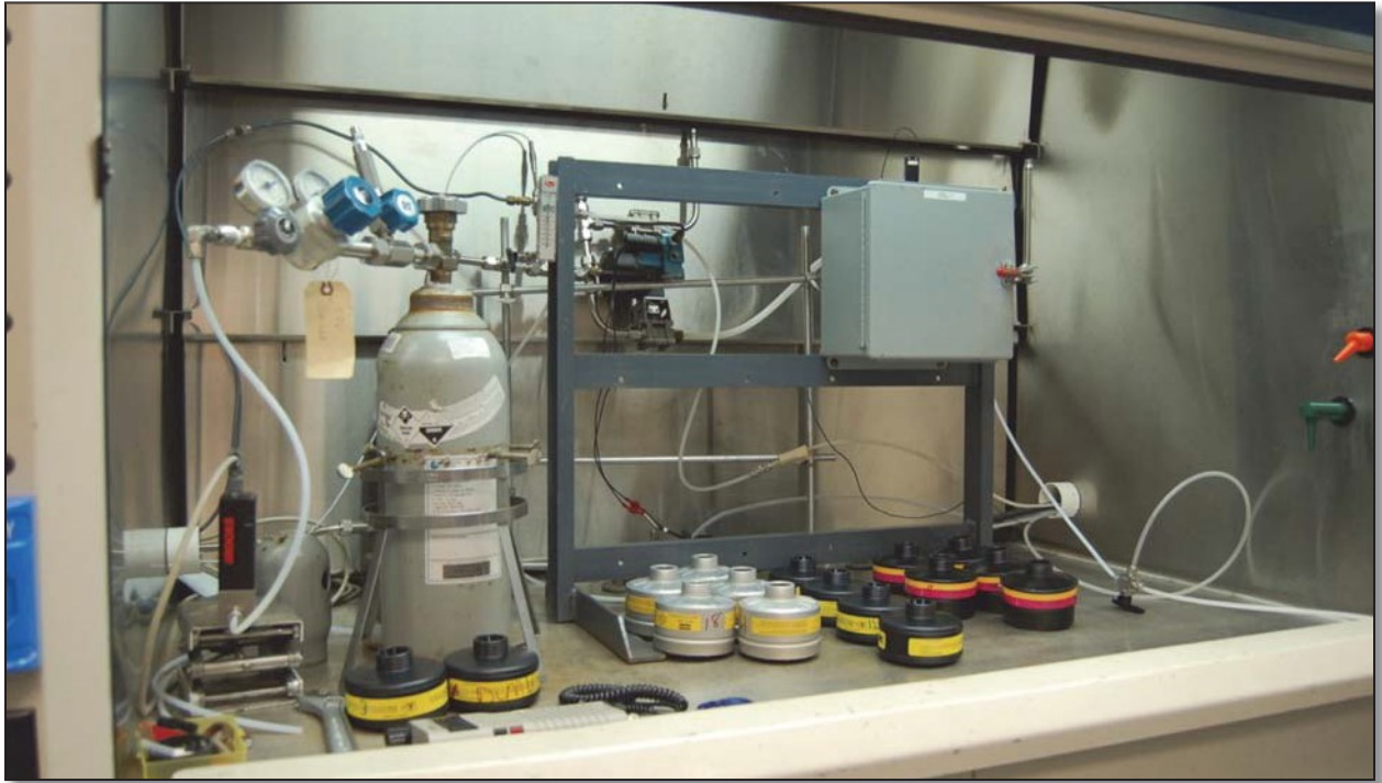
Figure 2-8. NIOSH Service Life Test Chamber
