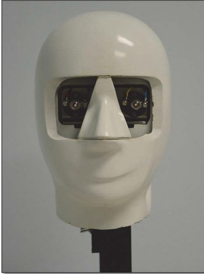
Figure 2-17. Stoll Apertometer Test Fixture
