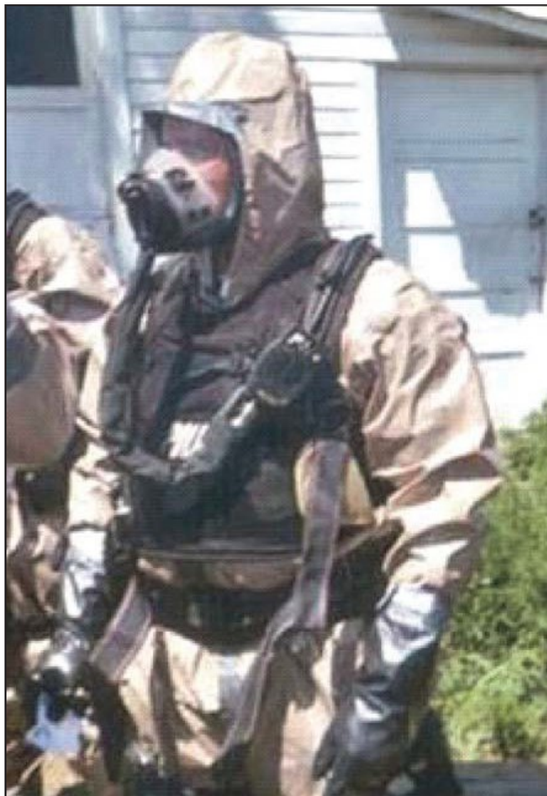
Figure 3-2. CBRN SCBA equipment used in an emergency response in which the contaminants are not known.
