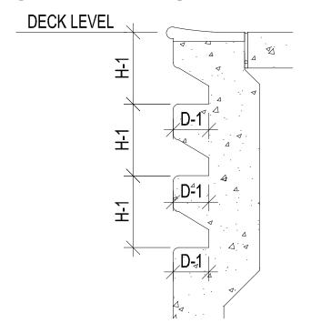
Figure 4.5.7.4.2: Recessed Step Dimensions: Front View
