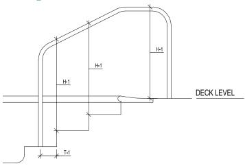
Figure 4.5.5.7.1: Stair Handrails: Side View
