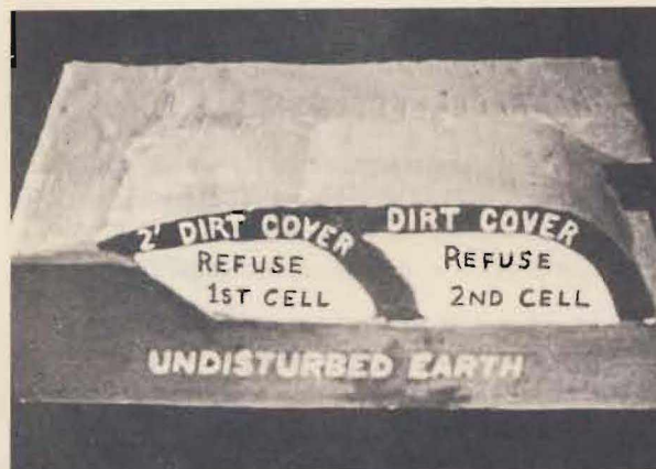
In a sanitary land fill, each day's collection of garbage should be compacted in a cell with a 2 foot cover of dirt.
