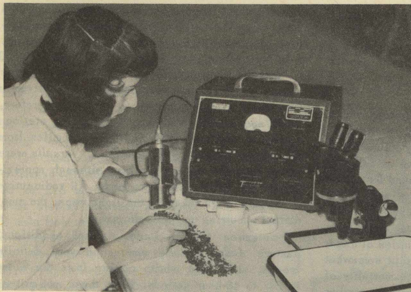
Figure 2. The Geiger counter was used to examine light trap collections for radioactive mosquitoes. (Photo courtesy Turlock Mosquito Abatement District and Lindblom Photo Service).
