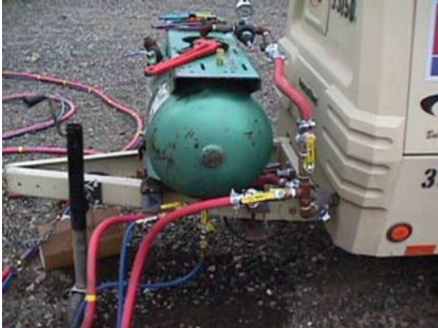
Figure 3. Water tank mounted on compressor trailer
