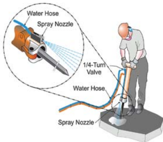
Figure 2. Diagram of water-spray control used in NIOSH study
