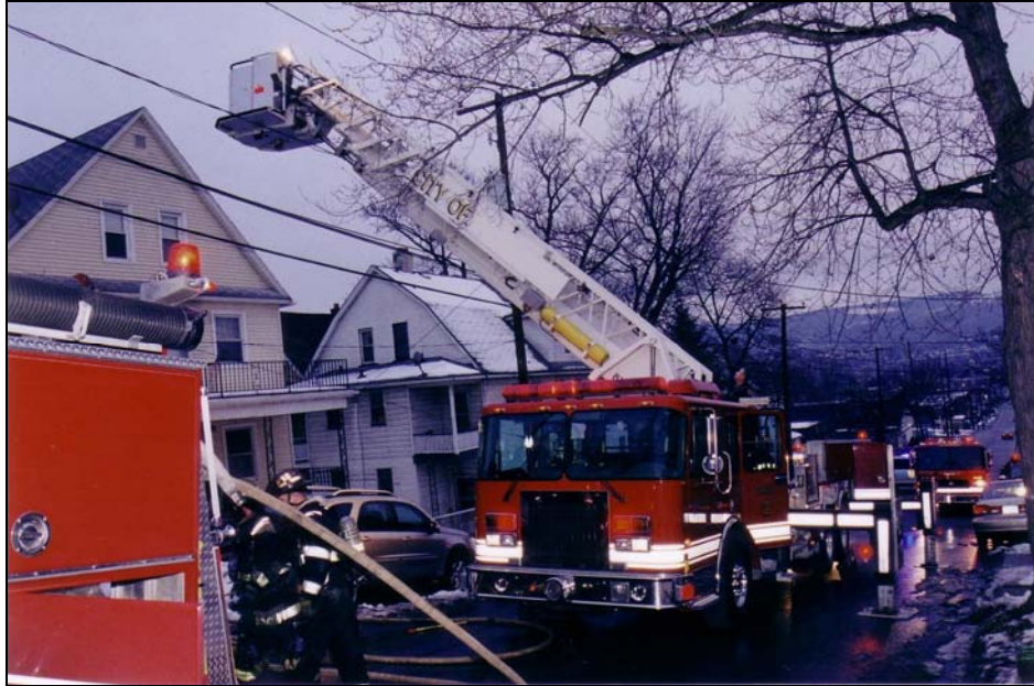
Photo 2. Truck 02 - 2002 model, 85-foot mid-mount, elevating platform. (Photograph taken shortly after the incident occurred by off duty fire fighter Bill Boock.)
