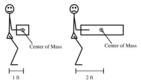
Figure 34.—Examples of holding a crib block. (A) With the crib block held by its sides, the distance from the spine to the center of gravity is 1 ft; (B) if held lengthwise, the center of gravity is 2 ft from the spine.
