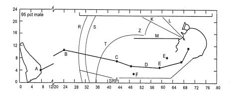
Figure 38.—Seating space envelopes for 95th-percentile miners in 42-in (top) and 22-in (bottom) compartments [Canyon Research Group 1982].
