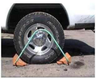
Figure 28.—Attaching a simple handle to wheel chocks greatly reduces excessive bending to place or remove the chocks [Torma-Krajewski et al. 2006].
