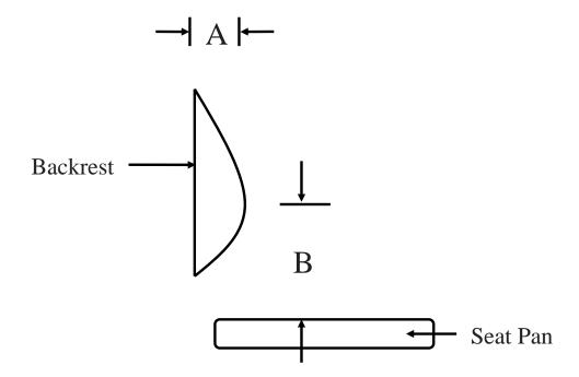
Figure 37.—Suggested dimensions for design of lumbar support. Maximum depth of the lumbar support (A) should be 0.6-0.8 in. The maximum convexity (B) should occur at a height of 9 in. above the seat pan. The seat should allow adjustment of these dimensions for proper fit.
