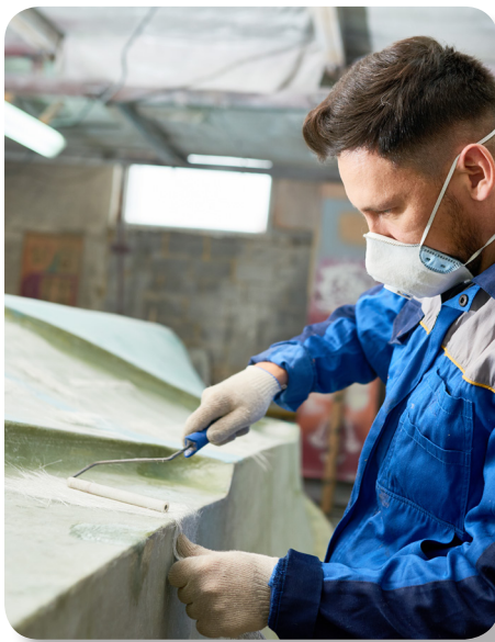
Incorrect respirator use due to beard and strap placement
