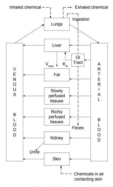
Note: This is a conceptual representation of a physiologically based pharmacokinetic (PBPK) model for a hypothetical chemical substance. The chemical substance is shown to be absorbed via the skin, by inhalation, or by ingestion, metabolized in the liver, and excreted in the urine or by exhalation.
