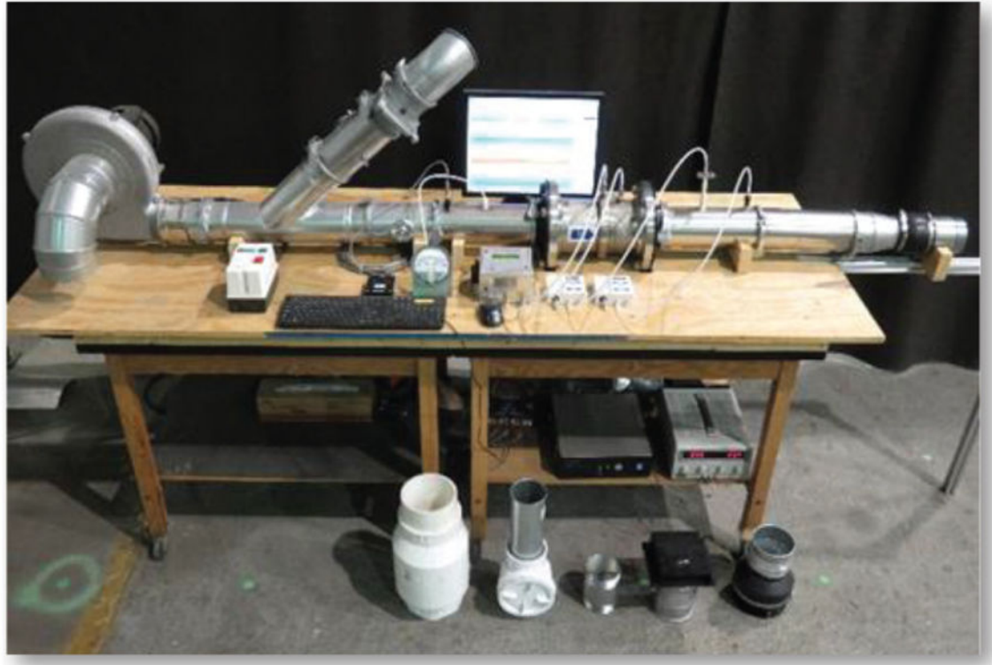
Figure 2. Pressure relief valve test stand (photograph).
