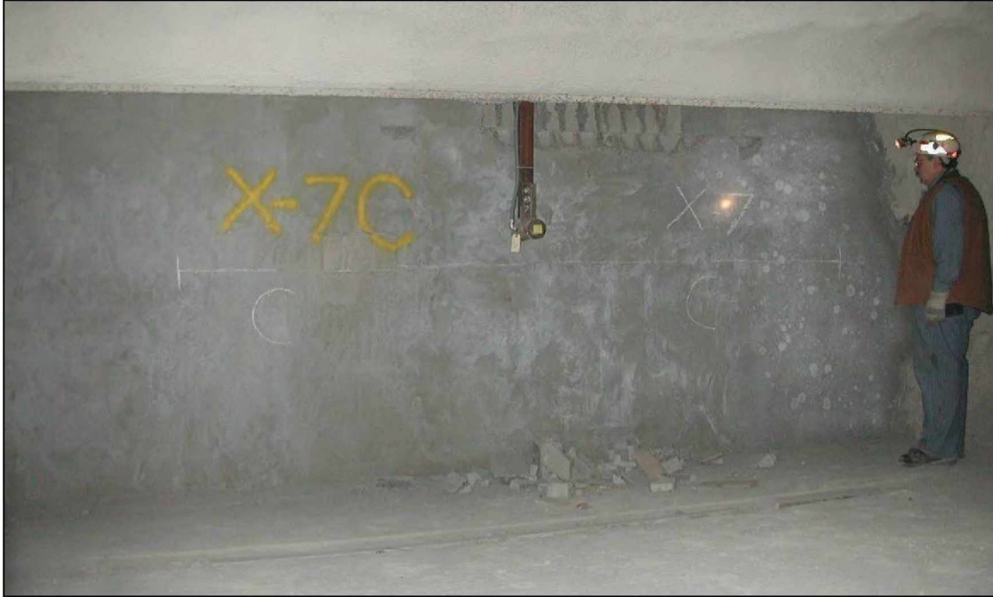
Figure 54.—Condition of X-7 dry-stacked hollow-core concrete block stopping after explosion test #433, viewed from C-drift side.
