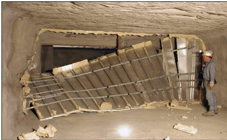
Figure 66.—Debris from steel panel stopping in X-7 after LLEM test #458, viewed from B-drift.
