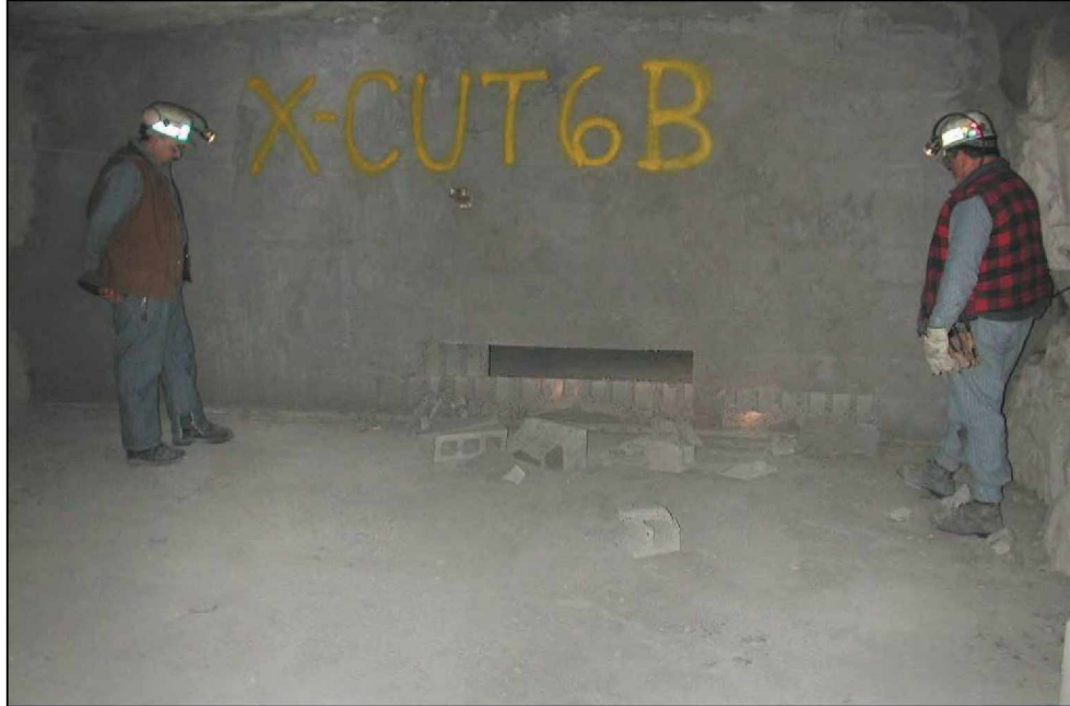
Figure 45.—Crosscut 6 dry-stacked hollow-core concrete block stopping viewed from B-drift side after LLEM test #430, showing blocks dislodged by explosion.
