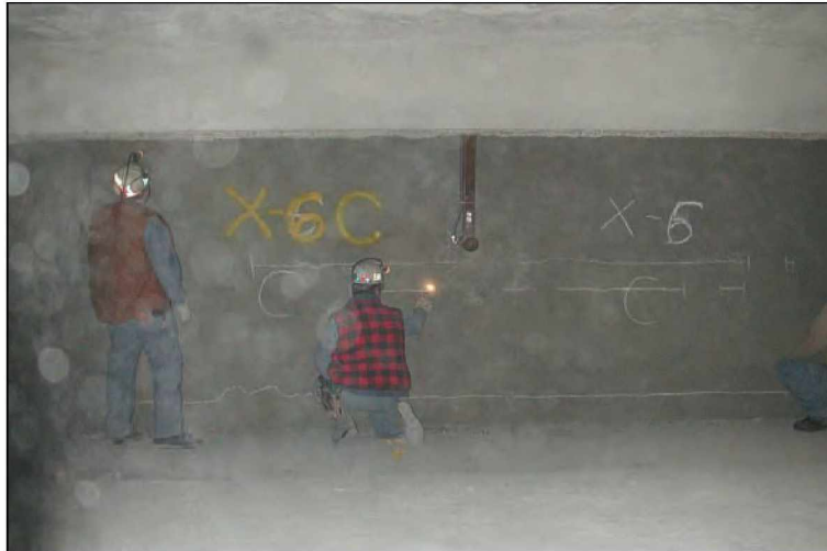
Figure 41.—Dry-stacked hollow-core concrete block stopping in X-6 remained intact after LLEM test #428. Chalk highlighted the cracks in the surface coating material.
