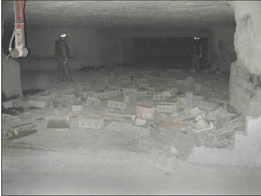
Figure 37.—Debris from X-5 dry-stacked hollow-core concrete block stopping after LLEM test #428, viewed from C-drift.
