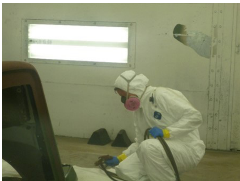
Figure 4. Employees spray painting a military vehicle part inside the spray paint booth. Photo by NIOSH.
