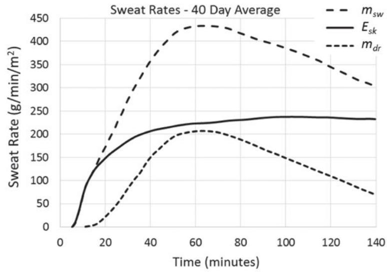
**Figure 3.** Transient total sweat and evaporated sweat rates showing effects of hidromeiosis (Candas, Libert and Vogt, 1983).
