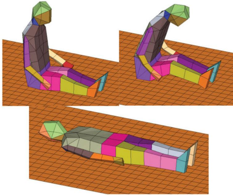
**Figure 2.** TAItherm modeling of three human poses: sitting with legs flat, sitting with legs bent, and lying.
